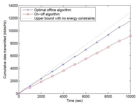
Improvement of optimal algorithm over an on-off transmitter in a simulation with truncated Gaussian arrivals.
