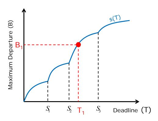
Optimal allocation for TCTM with  $B_I$ bits
