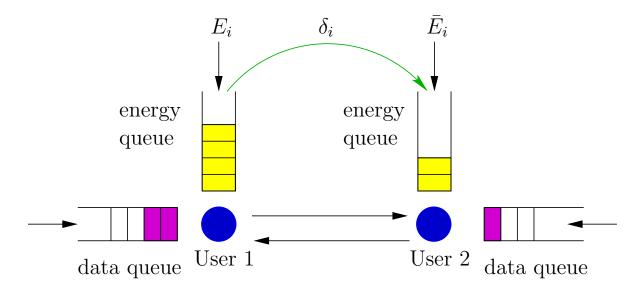
• Physical layer is a Gaussian two-way channel:
