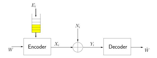
• Code symbols are constrained to the battery energy at each channel use:
