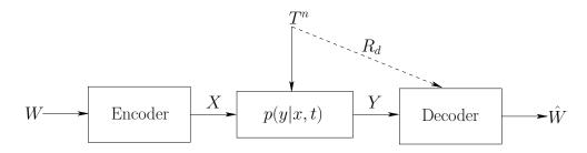
Figure 4.1: The state-dependent channel with rate-limited state information at the receiver.
