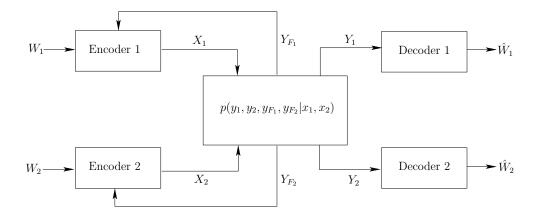
Figure 3.2: The interference channel with generalized feedback (IC-GF).
