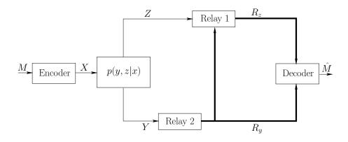
Figure 5.4: The diamond channel with partially separated relays.
