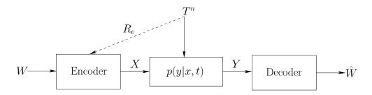
Figure 4.5: The state-dependent channel with rate-limited state information at the transmitter.
