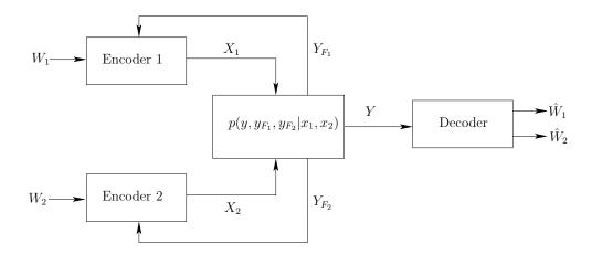
Figure 3.1: The multiple access channel with generalized feedback (MAC-GF).
