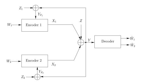
Figure 3.3: The Gaussian MAC with noisy feedback.
