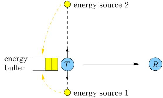
Fig. 1. Mobile energy harvesting node moving along a straight line.
