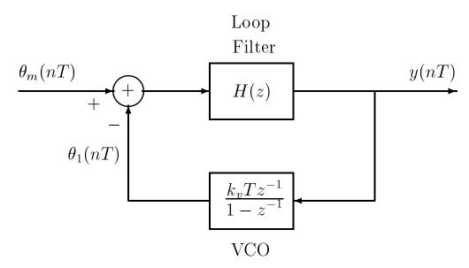
The transfer function for the linearized PLL is
