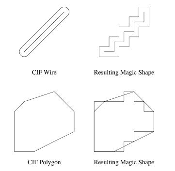
The shape of the Magic stairstep depends on the order in which vertices appear in the CIF or Calma file. The stairstep is made by first incrementing or decrementing the x-coordinate, then incrementing or decrementing the y-coordinate, then x, then y, and so on. For example, in the figure above, the polygon was specified in counter-clockwise order; if it had been specified in clockwise order the result would have been slightly different.
