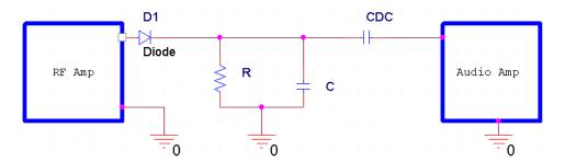
This type of demodulator is also called an "average envelope detector", and the conditions for good demodulation are as follows:
