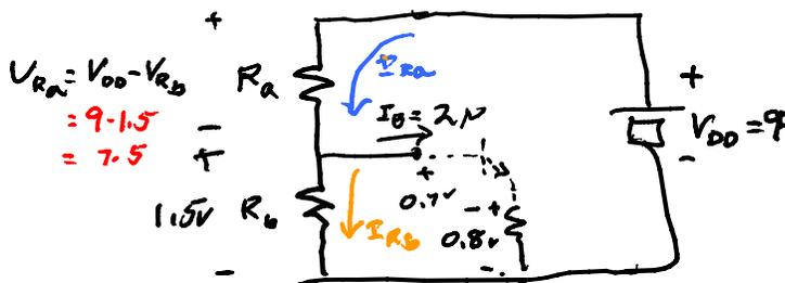
$$V_{R_a} = V_{DD} - V_{R_b}$$
