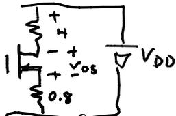
Choose  $V_{DD} = 9V$ ; need  $V_{GS} = 3.2$  so now design  $R_a, R_b$
