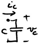
$$i_c = C \frac{dv_c}{dt} \quad \text{for bias } \frac{dv_c}{dt} = 0 \text{ as @ DC}$$
