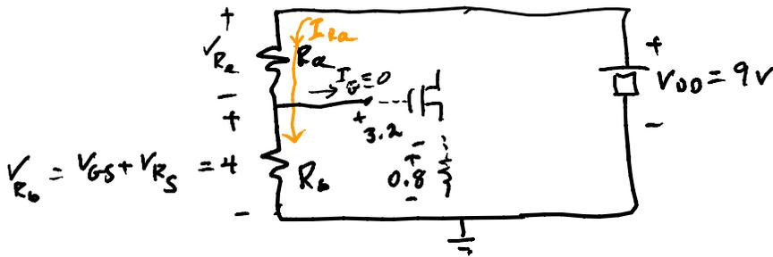
$$V_{R_b} = V_{GS} + V_{RS} = 4$$
