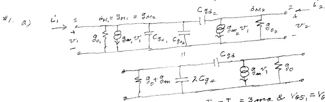
$$(Here g_{o1} = g_{o2}, g_{m1} = g_{m2} \text{ as } I_1 = I_2 = 3 \text{ mA} \text{ & } V_{GS1} = V_{GS2}) \quad \begin{matrix} C_{gd_2} \\ \oplus g_m v_1 \\ C_{gd_2} \end{matrix} \quad \begin{matrix} \oplus g_m v_1 \\ \oplus g_{o2} \\ \oplus g_{o1} \end{matrix} \quad \begin{matrix} \oplus g_{o1} \\ \oplus g_{o2} \end{matrix}$$
