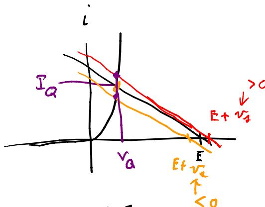
$$i_D = f(v_d) = I_D + \frac{df(v_d)}{dv_d} \Big|_{V_Q} (v_d - V_Q) + \frac{1}{2} \frac{df^2(v_d)}{dv_d^2} \Big|_{V_Q} (v_d - V_Q)^2 + \dots$$
