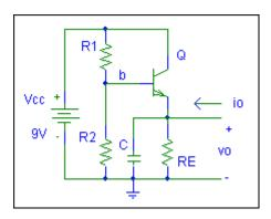
Assume the transistor has BF=199 and IE=-2mA, VA=100V, RE=1.15kOhm,  $C\pi$  = 0. Use VT=26mV and VBE=0.7V if needed..
