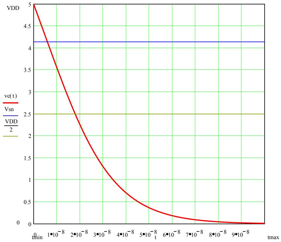
delay time,  $td$  = time to reach  $V_{\text{DD}}/2$ , which occurs in Ohmic region
