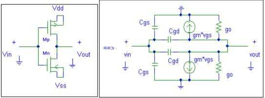
a) Combine all the parallel components of the equivalent circuit and draw the 2-port result. Then give the 2x2 admittance matrix Y(s) for the resulting 2-port.b) Note that the bias Vin=Vout=0 V. Determine the bias drain currents and the resulting gm and go.
