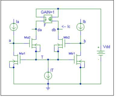
For the above circuit assume that all transistors are equal with W=L and when turned on are in saturation. Assume that a digital one is represented by I=1ma and a digital zero by I=0mA. Assume also the tail current IT=1mA and sufficiently large  $\lambda n$ .
