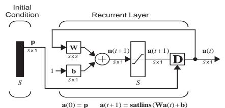
Note: The transfer function to be used is symmetric saturating linear function defined as
