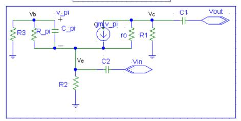
Above, is the small signal model of the circuit.
