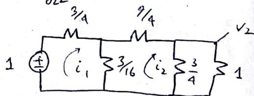
$$(c) \text{ Here, } \frac{v_2}{v_1} = \frac{k\lambda^2}{\lambda^4 + 3\lambda^3 + 8\lambda^2 + 9\lambda + 12} = \frac{\frac{k\lambda^2}{3\lambda^3 + 9\lambda}}{1 + \frac{\lambda^4 + 8\lambda^2 + 12}{3\lambda^3 + 9\lambda}}$$
