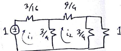
(d) For part (a),  $\frac{V_2}{V_1} = \frac{12}{s^4 + 3s^3 + 8s^2 + 9s + 12} = \frac{\frac{12}{3s^3 + 9s}}{1 + \frac{s^4 + 9s^2 + 12}{3s^3 + 9s}} = \frac{y_{21}}{1 + y_{22}}$
