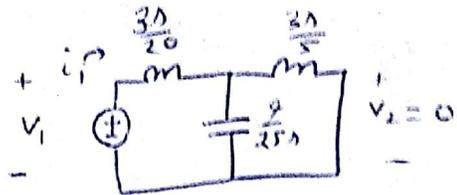
$$\begin{aligned} \text{Here, } Z_{11} &= \frac{3s}{20} + \left( \frac{9}{25s} \parallel \frac{3s}{5} \right) \\ &= \frac{3s}{20} + \frac{\frac{9}{25s} \times \frac{3s}{5}}{\frac{9}{25s} + \frac{3s}{5}} \\ &= \frac{3s}{20} + \frac{27s}{5(15s^2 + 9)} \end{aligned}$$
