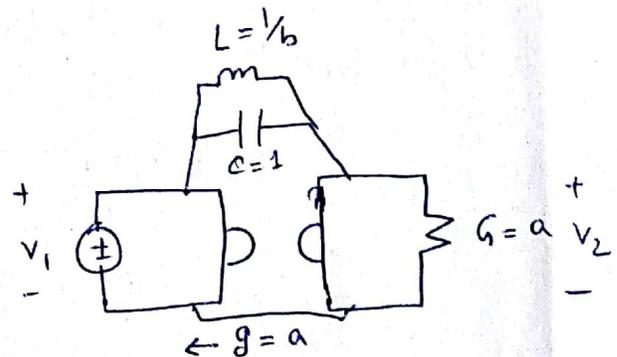
this is an all-pass constant-R circuit utilized via modified Richards' section.
