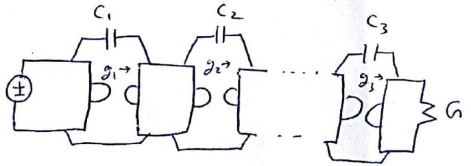
where,  $G_1 = 1$ , & for convenience, choose,  $g_1 = g_2 = \dots = g_n = 1$ , &  $c_1 = \alpha_1$ ,  $c_2 = \alpha_2$ ,  $\dots$ ,  $c_n = \alpha_n$ . Thus, any rational all-pass circuit can be easily synthesized via Richards' sections.
