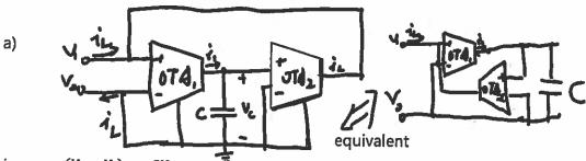
$$i_1 = g_{m1}(V_1 - V_2) = sCV_C$$
