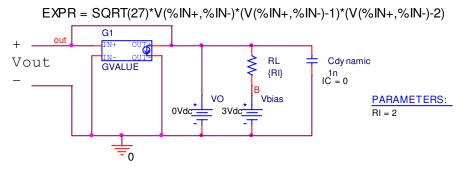
b) Remove VO and run a transient analysis and plot the current in the capacitor versus the voltage on the capacitor.
