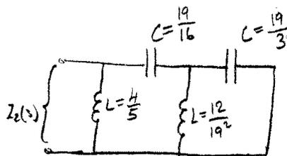
• Comparing the Cauer forms, we see that Capacitors and Inductors between  $y_1$  and  $y_2$  have been interchanged. Also, the leading component appears in parallel in  $y_2$  while it would be in series in  $y_1$ .
