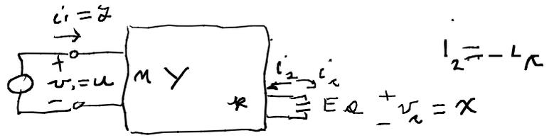
$$y_1 = i_1 = y_{11} v_1 + y_{12} v_2 = y_{11} u + y_{12} x$$
