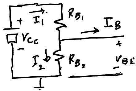
1) KCL:  $I_1 = I_B + I_2$ ,  $V_{BE} = R_{B2} I_2$ , Ohm's law
