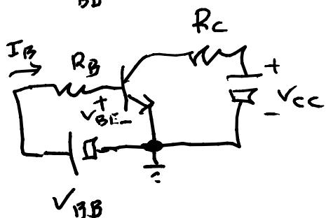
$$\Rightarrow 0 = -V_{BB} + R_B I_B + V_{BE} \quad \Rightarrow 0 = -V_{CC} + R_C I_C + V_{CE}$$
