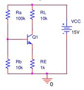
For the above circuit the transistor is a 2N3904. [the models in the ECE PSpice bipolar library seem to be in error; use those on the 303H web page]. The problem is to check its biasing.
