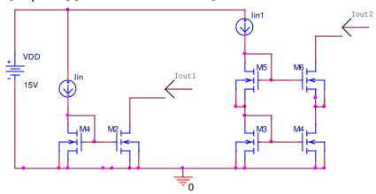
Here all transistors are 4007's and the problem is to show how the cascade current mirror is an improvement.
