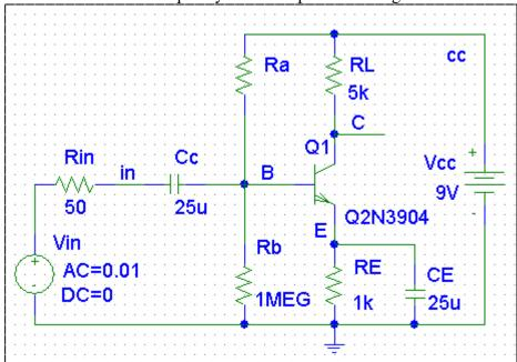
2. Using the following circuit find  $f_T$  for the above transistor at the bias point.
