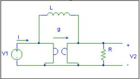
a) Draw the adjoint to the non-source portion of the circuit and set up sources on the adjoint in order to calculate the derivative of the transfer function V2/V1(s) with respect to the resistance R and also with respect to L. Calculate these derivatives using the adjoint and check by direct differentiation of the transfer function.
