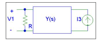
3. Give the conditions on the transfer function T(s)=V1/I2 for it to be realizable when the 2-port for Y(s) is a lossless ladder and when R>0. What changes if the 2-port is lossless but not restricted to be a ladder? What if R<0 is allowed?
