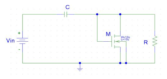
4. Using the results from 3, give the semi-state variable descriptions and equations of the circuit. Use the capacitor voltage as the state and the voltage-current vector as the semi-state variables. Use the source as the input and the capacitor voltage as the output.
