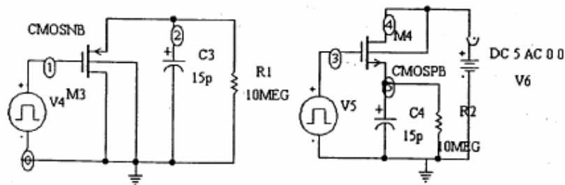
For nmos,  $t_{PLH} \approx 8k\Omega \times 15pF = 120\text{ns}$ ; for pmos,  $t_{PLH} \approx 360\text{ns}$
