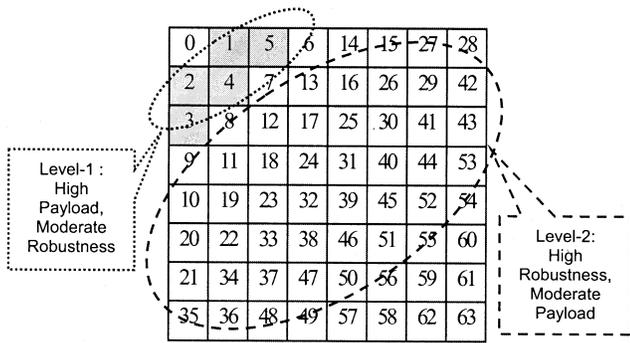
Fig. 2. Spectrum partition of two-level data hiding in block-DCT domain.
