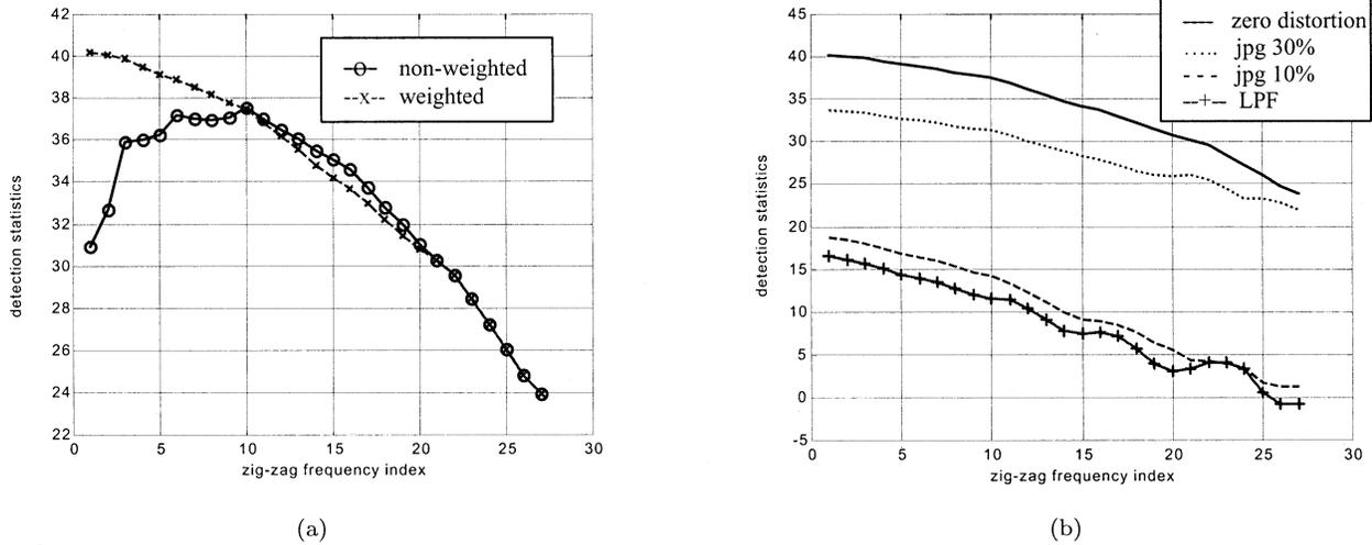
Fig. 1. Average detection statistics: (a) detection statistics of nonweighted correlator  $q$  (circles) and of weighted correlator  $q'$  (crosses) with no additional distortion and (b) detection statistics of weighted correlator  $q'$  under four different distortions. The  $x$ -axis in both plots indicates the frequency band in a zigzag order from which watermark starts to be put in.
