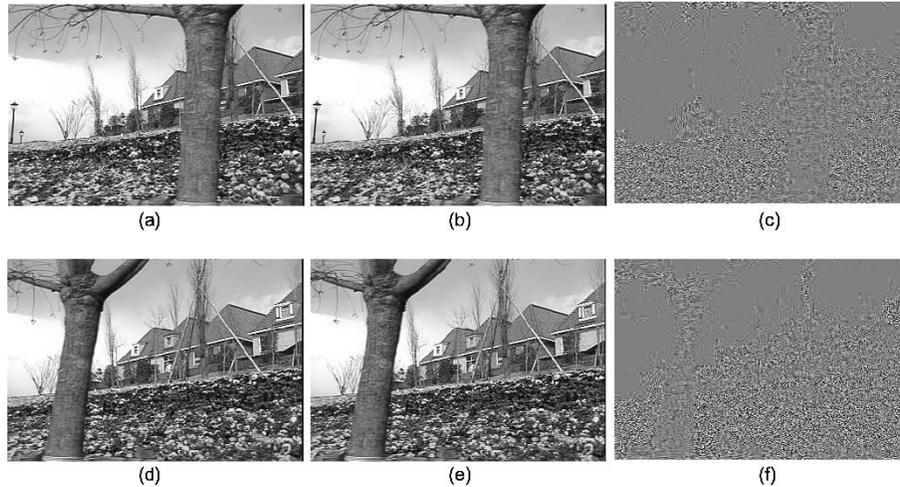
Fig. 8. Multilevel data hiding for the flower garden video sequence: (a) the original 1st frame, (b) the watermarked 1st frame, (c) the amplified difference of (a) and (b); (d) the original 30th frame, (e) the watermarked 30th frame, and (f) the amplified difference of (d) and (e). The video is compressed with MPEG-2 at 4.5Mbps, and the differences are amplified by a factor of 5 with gray denoting zero difference and black/white denoting large difference.
