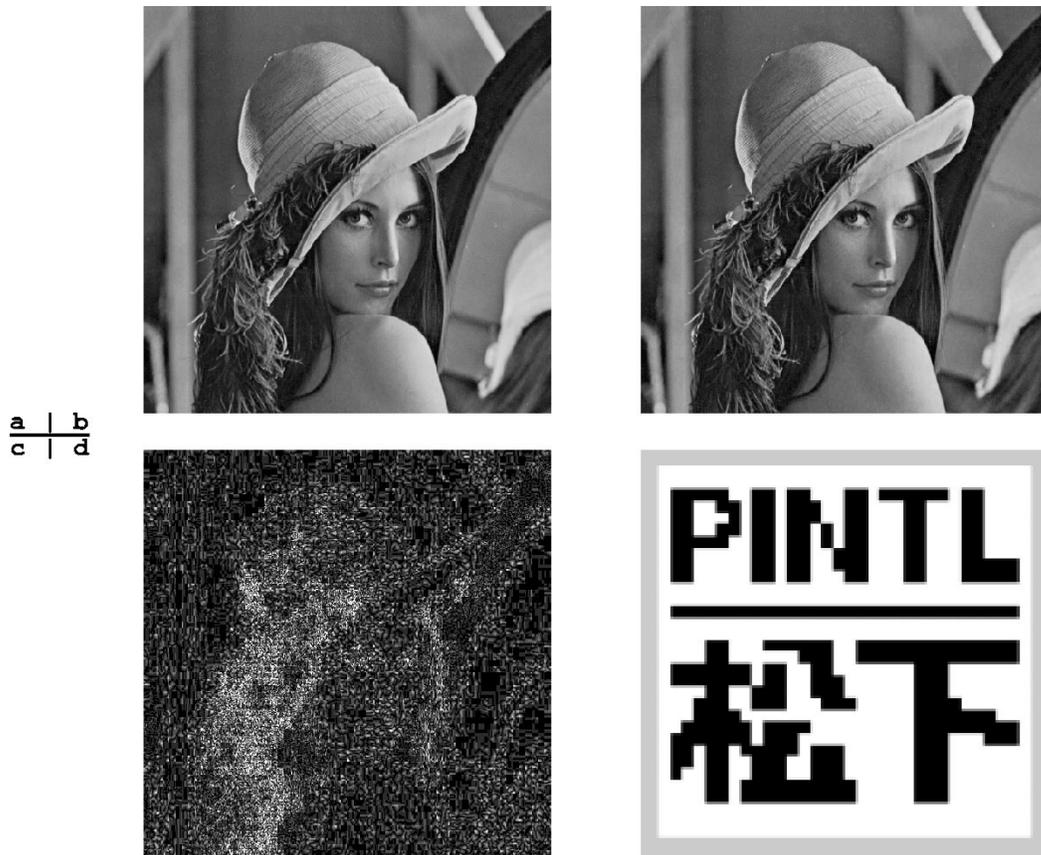
Fig. 4. Multilevel data hiding for Lenna image ( $512 \times 512$ ). (a) original image; (b) watermarked image; (c) amplified difference ( $\times 5$ ) between (b) and (a) with black denoting zero difference; and (d) extracted  $32 \times 32$  PINTL-Matsusita logo from the low band.
