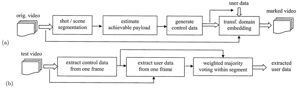
Fig. 7. Block diagram of the proposed video data hiding system: (a) embedding process and (b) detection process.
