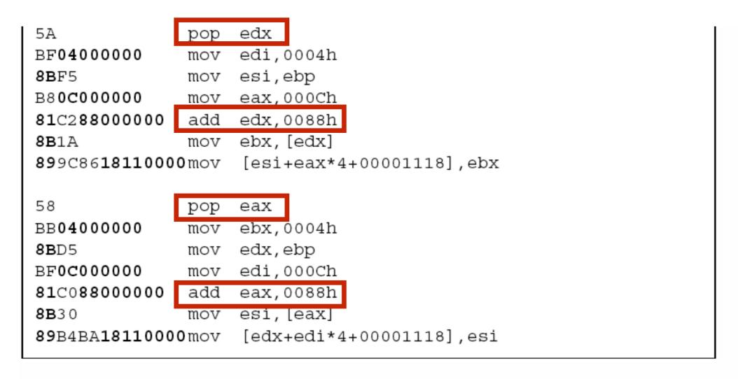
Figure 4: Win95/Regswap using different registers in new generations
