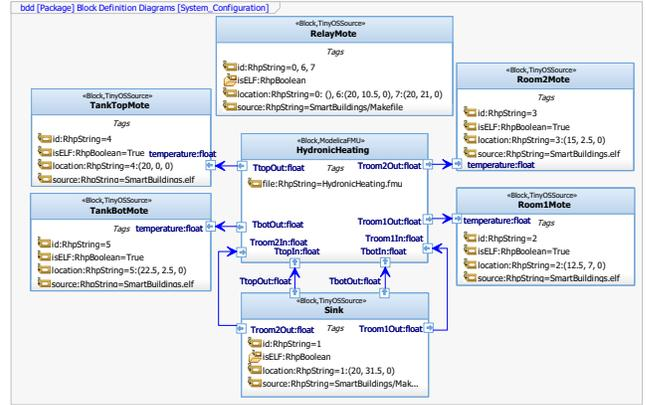
Fig. 3. System Configuration
