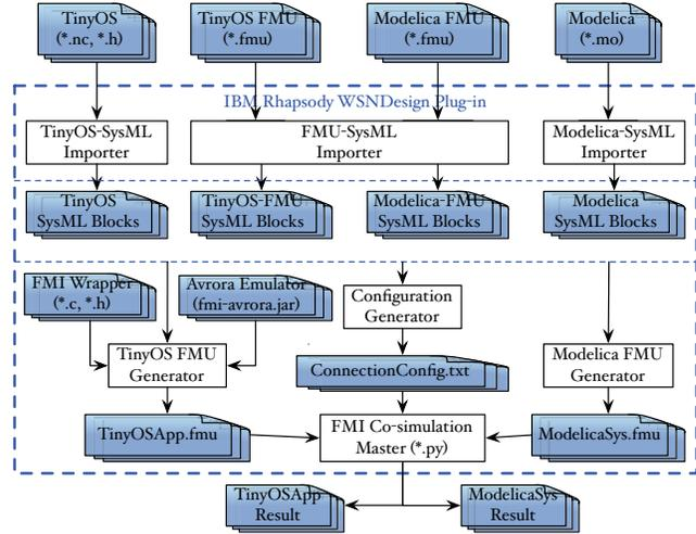
Fig. 1. HybridSim Toolchain Workflow
