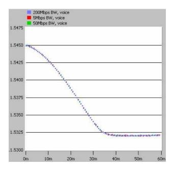
Figure 4. End-to-end voice application delay (seconds)
