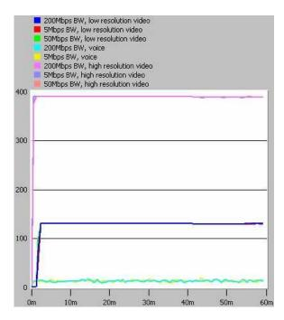
Figure 7. Satellite link throughput (packets/second)
