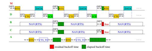
Figure 4: Nodes M and D collude and select a very small backoff, thereby denying access to node A by causing CTS timeouts.
