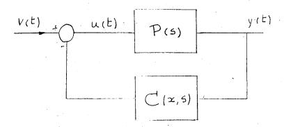
Figure 1. Standard multivariable control loop
