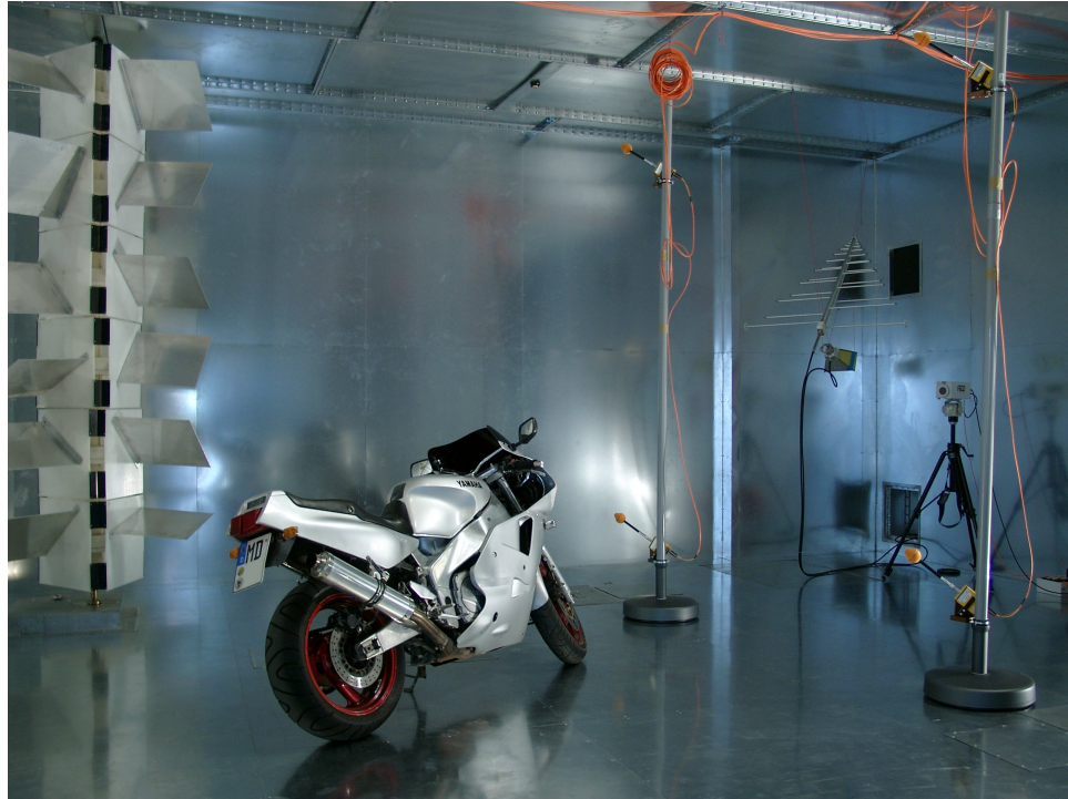
Figure 4.2: A example of a reverberation chamber at the Otto-von-Guericke-University Magdeburg, Germany, where electronic devices are test for immunity to high power electromagnetic sources [43]
