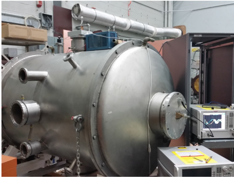
Figure 3.5: The cylindrical stainless steel enclosure with a rotating mode stirrer.
