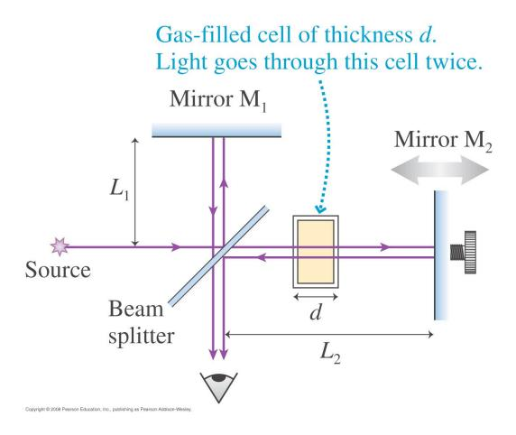
Number of fringe shifts as cell fills up Number of wavelengths in cell when empty
