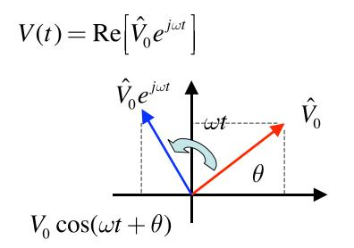
Multiplying  $\hat{V}_0$  by  $e^{j\omega t}$ rotates the angle of the product by  $\omega t$
