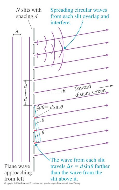
Diffraction Grating N slits, sharpens bright fringes
