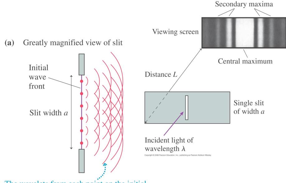
The wavelets from each point on the initial wave front overlap and interfere, creating a diffraction pattern on the screen.
