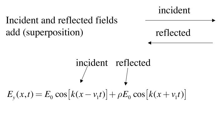
Incident and reflected waves will interfere, changing the peak electric field at different points
