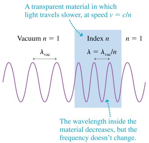
For sinusoidal waves the following is still true  $f\lambda = v_{em}$
