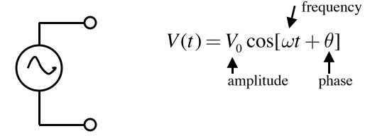
Examples: our power grid when it is on. f=60 Hz, V=110 V (RMS) audio signals communication signals Power in microwave ovens Power in MRI machines
