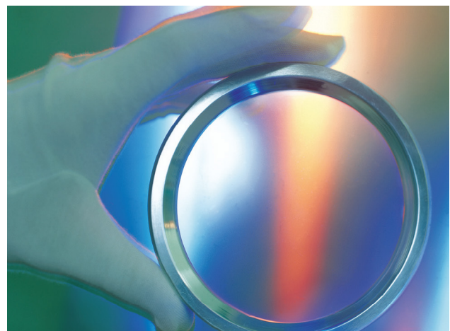
Microwave CVD diamond components have a transmission spectrum from 220 nm up to >50 \mu\text{m} . They also conduct heat better than any other material.
