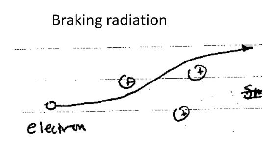
As charged particles (usually electrons) slow down in matter they are accelerated both longitudinally and transversely.
