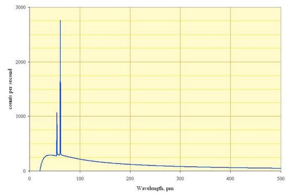
Spectrum of the X-rays emitted by an X-ray tube with a rhodium target, operated at 60 kV. The smooth, continuous curve is due to bremsstrahlung, and the spikes are characteristic K lines for rhodium atoms. - Wikipedia
