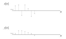
Filter acts on the input sequence  $x[\,\cdot\,]$  to produce the output sequence  $y[\,\cdot\,]$  , according to the equation
