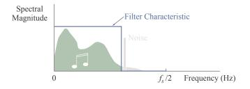
Filtering out noise from samples of an audio signal.
