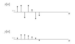
Filter acts on the input sequence  $x[\,\cdot\,]$  to produce the output sequence  $y[\,\cdot\,]$  , according to the equation
