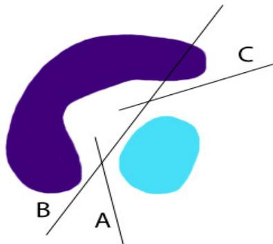
Fig. 4. Demonstration of how planes can be used to separate data. Here the relationship of a data point with the lines A, B and C determines whether the point is a member of either the blue or purple groups.
