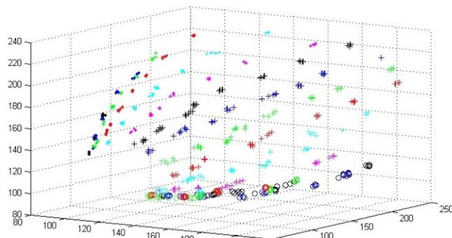
Fig. 1. Training data for 17-angle system. Different colors/markers represent different angles; clusters show different ranges. The axes are the amplitude values from the pingers. Units are arbitrary amplitude units.
