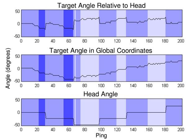
Fig. 9. Behavior of the 15-angle system when tracking an object for 200 pings. Background color indicates which pinger is firing: light blue represents left pinger, medium blue represents middle pinger, dark blue represents right pinger.
