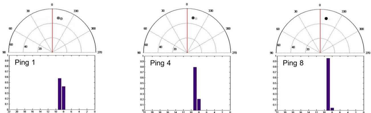
Fig. 11. Demonstration of how merging looks improves the certainty of observed objects. The top plots map the position of an object. A darker point indicates higher certainty. The lower plots are bars of the normalized output for the object. Data was collected from sonar using the 15-angle system.
