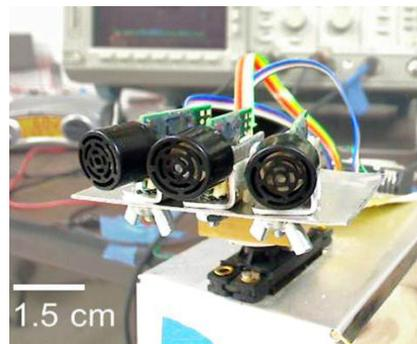
Fig. 1. Arrangement of the pingers on the rotational sonar head.
