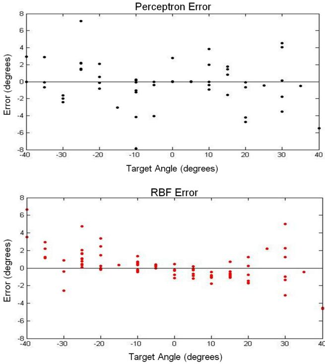
Fig. 7. Error of Perceptron learning algorithm (top) and RBF learning algorithm (bottom) for a subset of the 17-angle training data. Error is the difference between the calculated angle and the actual target angle.
