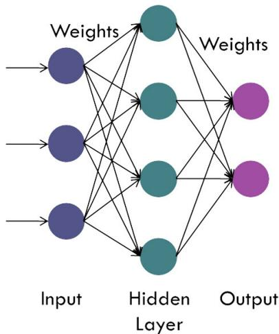
Fig. 2. Perceptron neural network diagram.
