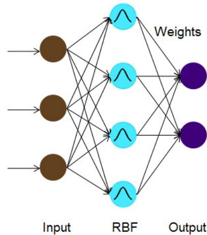
Fig. 5. Radial basis function neural network diagram.
