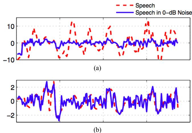
Fig. 3. Short-time power plots of a single mel-channel for (a) temporal difference over the logarithmic power of a speech signal (reflecting DCC) and for (b) the Gaussianization operation over the temporal difference of a speech signal (reflecting DSCC) [3].
