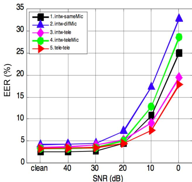
Fig. 1. Equal error rates of a speaker recognition system with an MFCC front-end in different levels of white noise [1]. Line colors indicate conditions for training and testing data according to the NIST 2008 SRE evaluation conditions: “intw-sameMic” indicates that data contained interview speech recorded on the same microphone in training and test; “tele-tele” indicates that telephone speech was used in both training and test [4].
