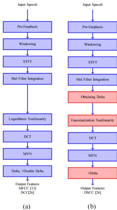
Fig. 2. Different extraction processes for (a) 13-dimensional MFCC features and 26-dimensional delta-cepstral coefficients (DCC), (b) 26-dimensional delta-spectral cepstral coefficients (DSCC) [3].
