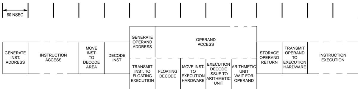
We'll assume for the moment that the fixed-point pipeline is similar to the floating-point pipeline, as is suggested by the general flow shown in figure 2. Here is the behavior of four instructions in
