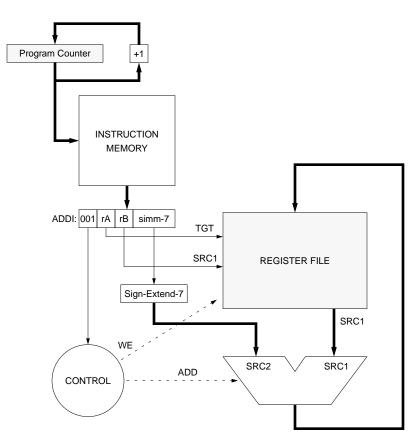
This figure illustrates the flow-of-control for the ADD IMMEDIATE instruction. Only two ports of the register file are used; the second source operand comes directly from the instruction word. The write-enable bit is set for the register file. The ALU control signal is a simple ADD function.
