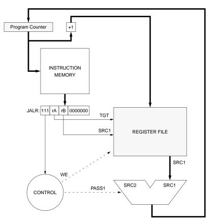
This figure illustrates the flow-of-control for the JUMP-AND-LINK-THROUGH-REGISTER instruction. This function uses two of the register file's three ports. A value is read from the register file and placed directly into the program counter, and the sum
