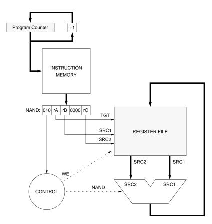
This figure illustrates the flow-of-control for the BITWISE NAND instruction. All three ports of the register file are used, and the write-enable bit is set for the register file. The ALU control signal is a BITWISE NAND function.
