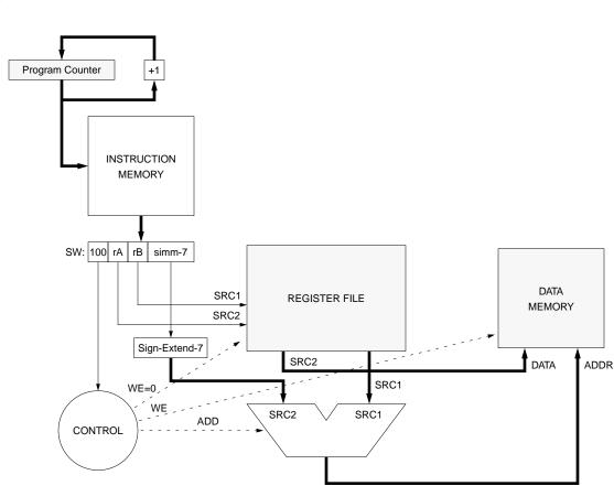
This figure illustrates the flow-of-control for the STORE DATA WORD instruction. Only two ports of the register file are used; the register file's write port (TGT) is not used. The SRC2 output port does not feed the ALU (as it normally does), but rather the DATA input of data memory. This is the value to be written to memory. The second ALU input is an immediate value that comes directly from the instruction word.
