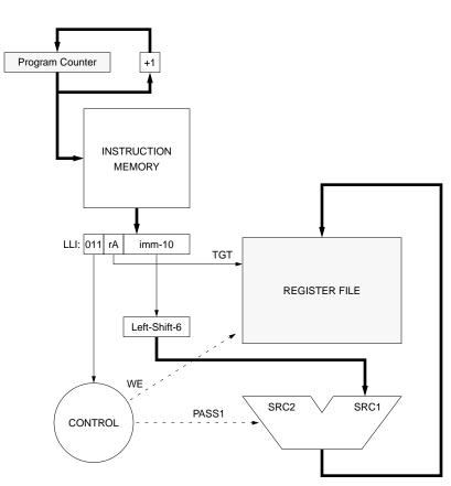
This figure illustrates the flow-of-control for the LOAD UPPER IMMEDIATE instruction. This instruction replaces the top ten bits of an instruction with ten bits found in the instruction word and zeroes out the bottom six bits. Only one port of the register file is used—the write port—as all of the bits destined for the register file are zero or come directly from the instruction word. The write-enable bit is set for the register file.
