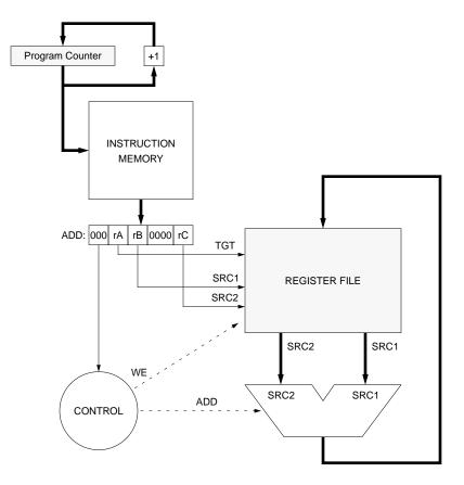
This figure illustrates the flow-of-control for the ADD instruction. All three ports of the register file are used, and the write-enable bit (WE) is set for the register file. The ALU control signal is a simple ADD function.
