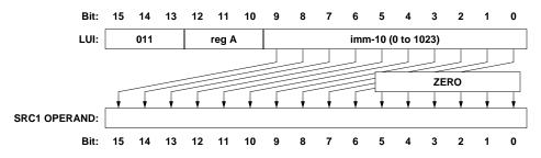
The second argument to the ALU (SRC2) is ignored; this is accomplished by setting the ALU control to be PASS1, which sends through the first argument unchanged. This same ALU control will be used for the JALR instruction as well. One could alternatively zero-extend the immediate value and use a SHIFT input to the ALU while inputting the value '6' at the other ALU-input. However, the illustrated mechanism seems slightly less complicated.
