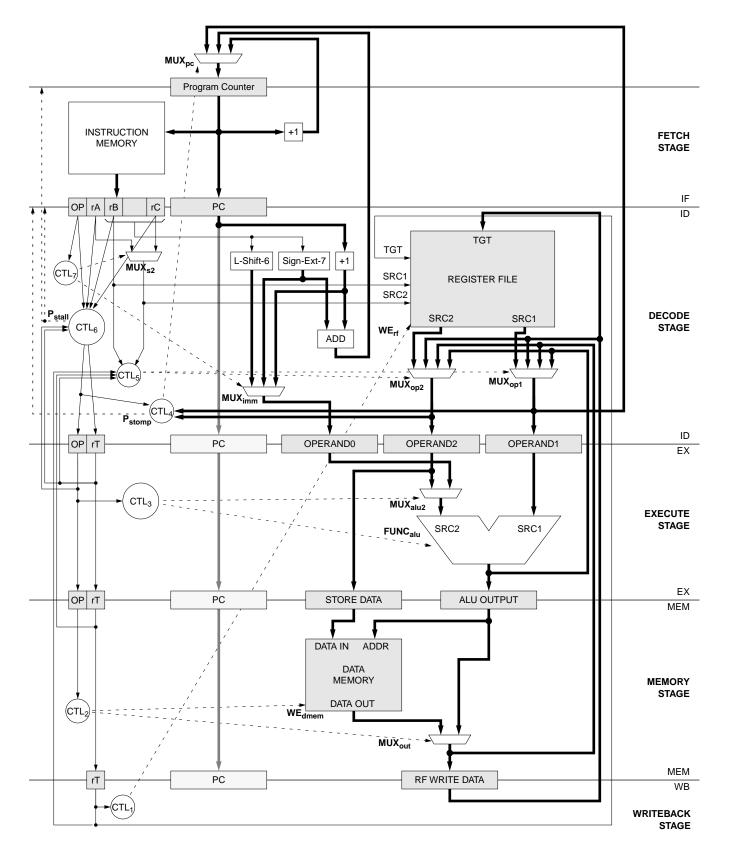
Fig. 1: RiSC-16 5-stage pipeline
