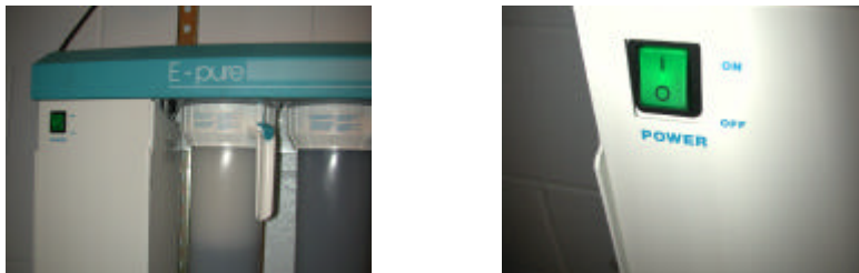
Fig 3. The green button at the low left side of E-pure is the power button.
