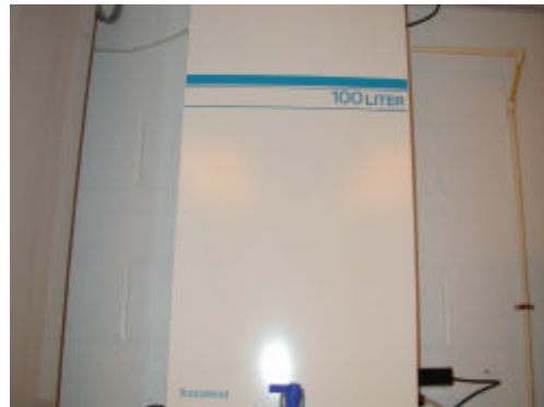
Fig 2. The E-pure water purification unit. It is hanging on the wall between the two fume hoods.
