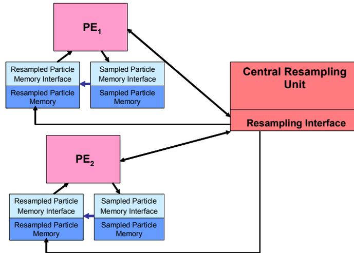
Figure 33. Distributed particle filter architecture.
