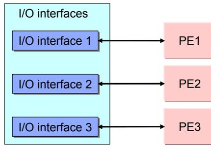
Figure 25. 3-PE architecture for error generation actor of speech compression application.
