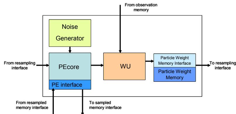
Figure 34. Single PE architecture.
