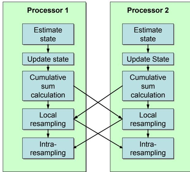
Figure 28. 2-PE architecture for fault detection system.
