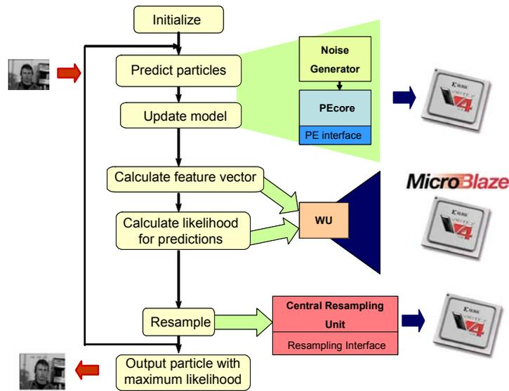
**Figure 37.** Mapping of subsystems of 3D facial pose tracking system onto hardware and software modules.
