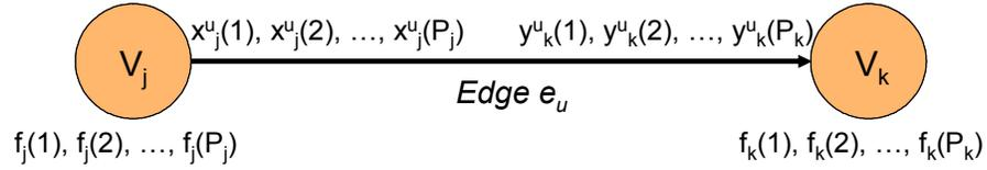
Figure 3. Example of a 2-actor CSDF graph.
