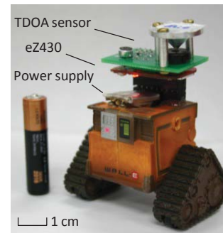
Fig. 1. Miniature robot platform. AAA battery shown for reference.
