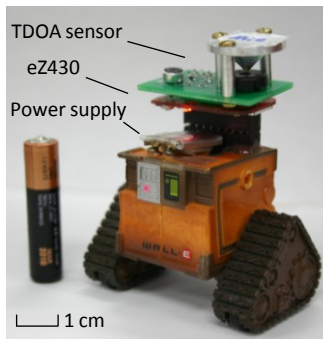
Fig. 1. Miniature robot platform used in the experiments. AAA battery shown for reference.
